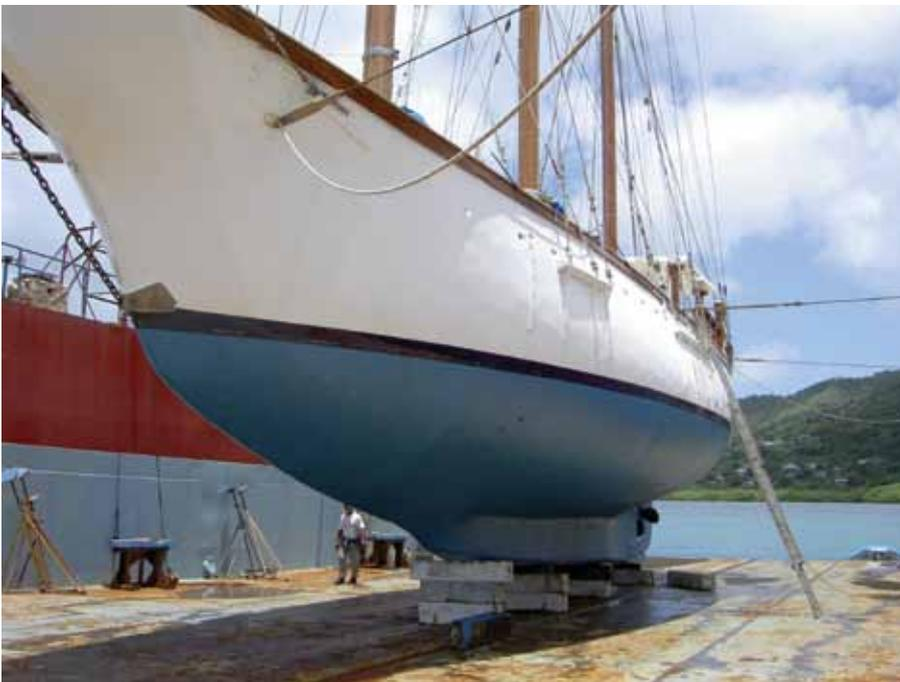
Fig. 6: The finished hull after epoxy coating and polyurethane application
