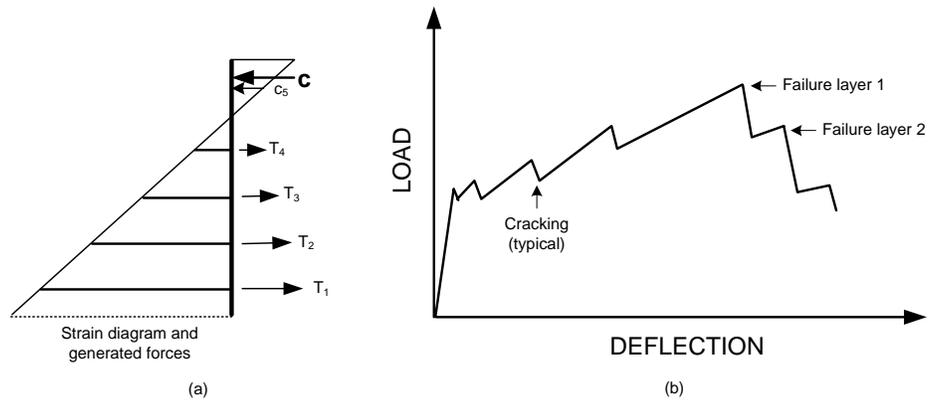
Figure 5 – Typical strain compatibility diagram for ferrocement plates reinforced with high performance FRP meshes and effect on load deflection response.
