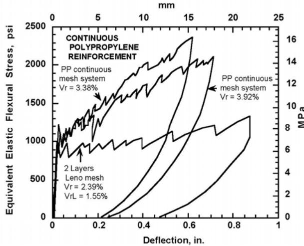
Figure 2 – Typical response of ferrocement plates reinforced with low modulus polymeric meshes
