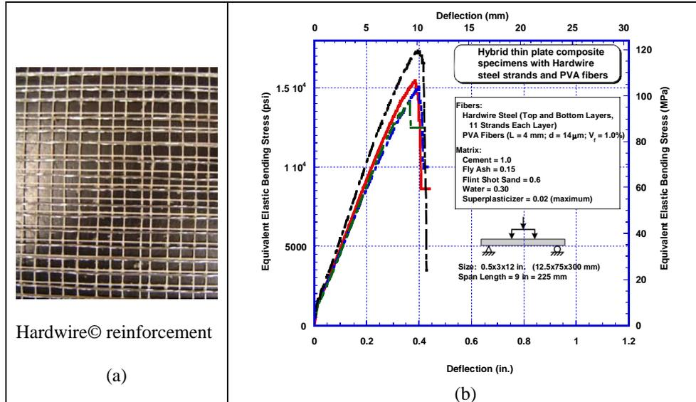
Figure 1 – Equivalent elastic bending stress versus deflection response of ferrocement plates reinforced with Hardwire© reinforcement
