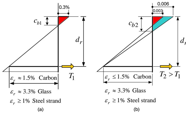
Figure 6 – (a) Typical strain diagram for balanced conditions using a plain mortar matrix. (b) Typical strain diagram illustrating the effect of doubling the strain capacity in compression by addition of fibers
