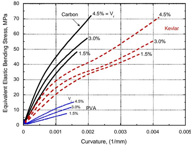
Figure 3 – Analytically predicted bending response of ferrocement plates reinforced with FRP meshes [53]
