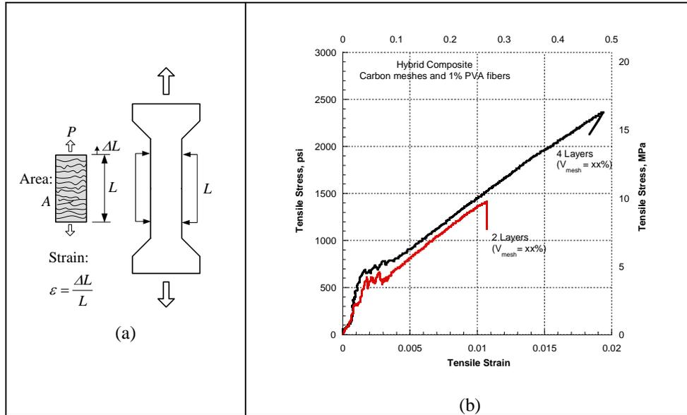
Figure 4 – Tensile stress-strain response of thin hybrid cement composites reinforced with carbon meshes and PVA fibers
