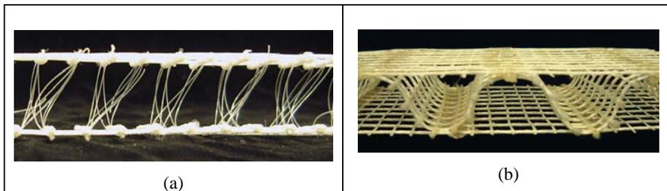
Figure 9 – Examples of three-dimensional (3D) mesh systems with FRP (textile) reinforcements fabricated at the ITA in Aachen, Germany: a) 3D spacer-sandwich textile; b) 3D spacer stiff textile
