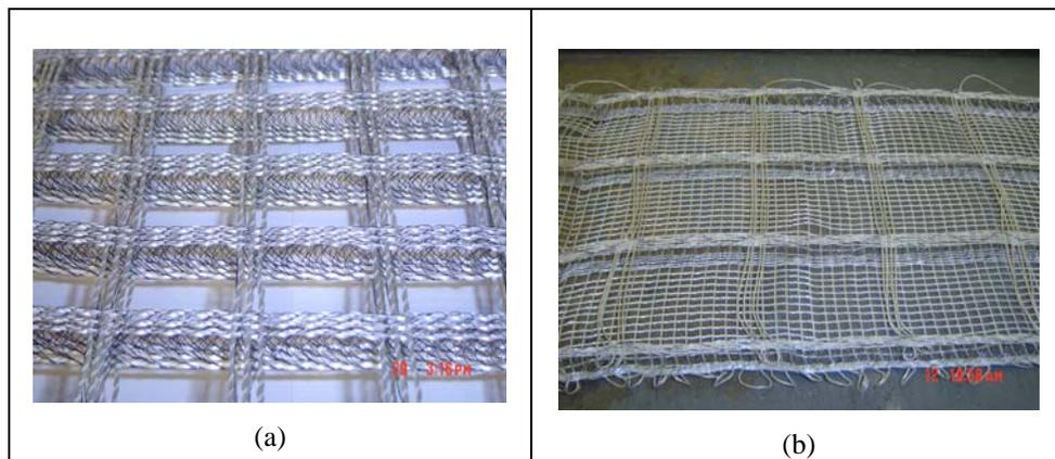
Figure 10 – Examples of three-dimensional (3D) mesh systems with FRP reinforcements fabricated at the ITA in Aachen, Germany: a) 3D ribbed textile; b) 3D joist-type textile
