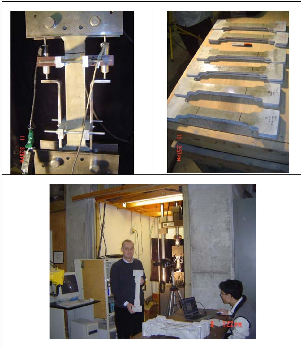
Tensile testing of ferrocement and FRC composites at the University of Michigan
