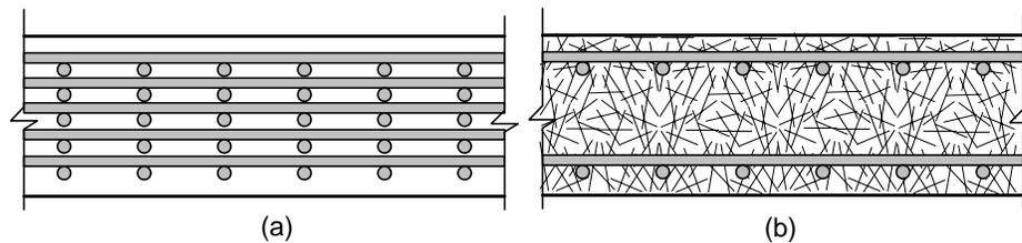
Figure 7 – (a) Typical section of ferrocement with several layers of mesh. (b) Typical section of efficient FRP hybrid composite with only two extreme layers of mesh and fibers
