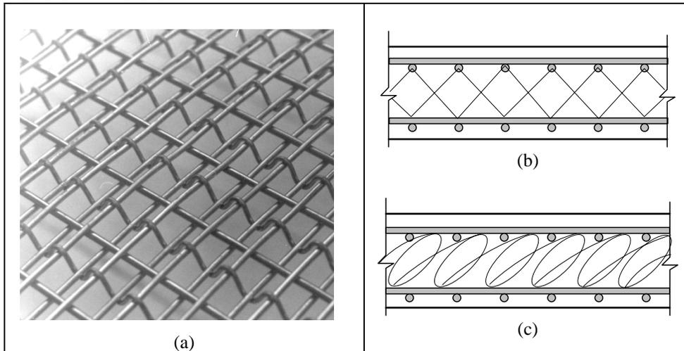
Figure 8 – Examples of three-dimensional (3D) mesh systems with steel reinforcement: a) Watson mesh [12]; b) Two square steel meshes joined by welded links [61]; c) Two square steel meshes joined by coiled links
